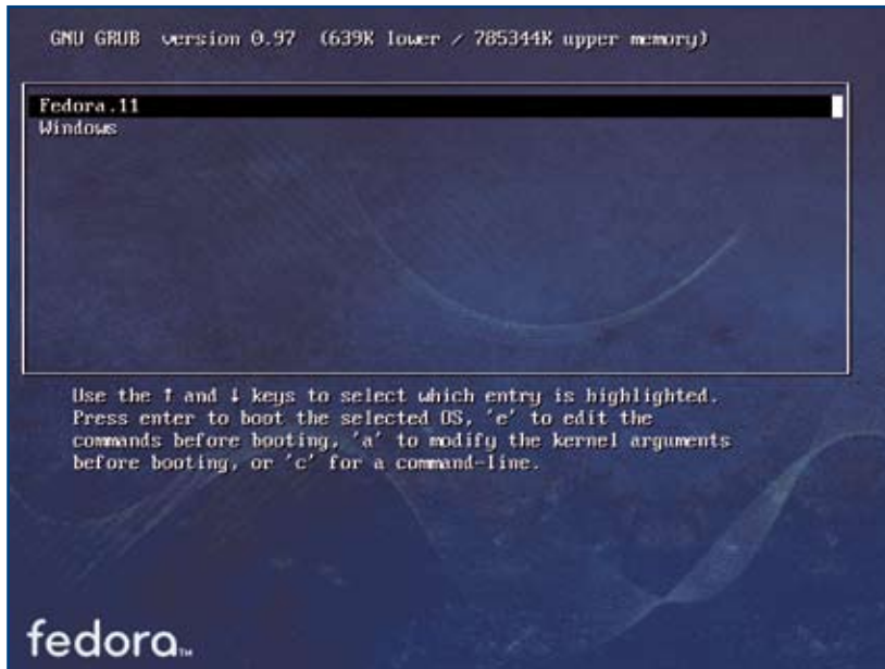
Figure 6. The GRUB menu allows you to choose what OS you want to boot into
